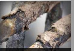
Typical hot water heater: Water comes in contact with extreme temperatures and causes scale build-up to form and ultimately product failure.
